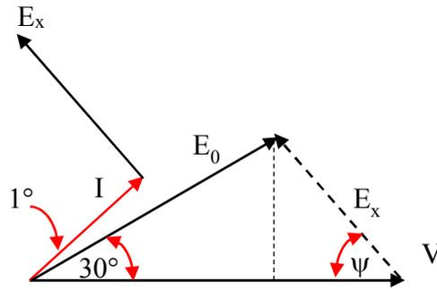
$$E_x = \sqrt{(V - E_0 \cos 30^\circ)^2 - (E_0 \sin 30^\circ)^2} = 7 \text{ kV}$$
